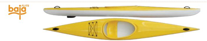
Max Capacity: 200lbs/90.7kg, Length 14 Ft (4.25m) Width 23.5 inches (60 cm), Boat weight: 35 lbs/15.8kg, Skeg Depth 1.75 inches (46mm)
