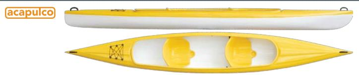
Max Capacity: 370lbs/167.7kg, Length 16 Ft (490 cm) Width 30 inches (77 cm), Boat weight: 55 lbs/24.9kg
